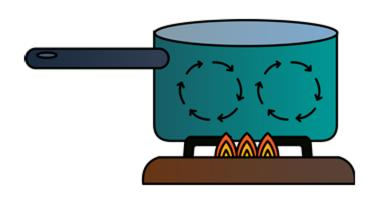
When you boil water in a pot, the water near the burner gets hot and becomes less dense. It rises up and pushes the cooler water out of the way. That cooler water sinks, gets heated, becomes less dense, and rises up. This creates a convection current.
